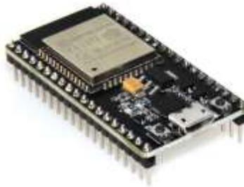
**Gambar 3.** Modul ESP32
