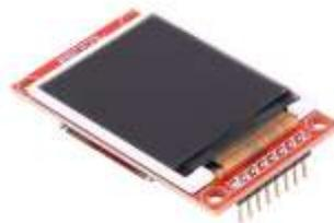
**Gambar 6.** LCD TFT 1.8
