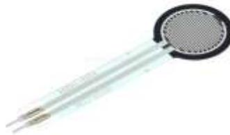
**Gambar 4.** Sensor FSR
